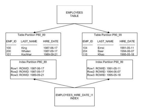
Figure 6-1. Locally partitioned index architecture
