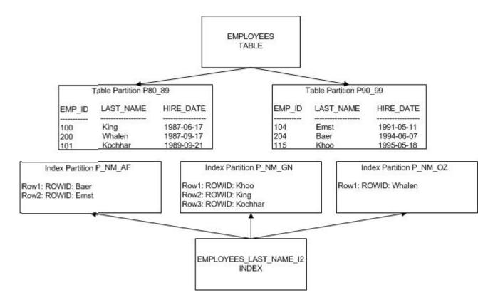
*Figure 6-2. Globally partitioned index architecture*
