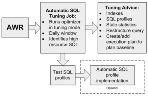
*Figure 9-1.* Architecture of the automatic SQL tuning job
